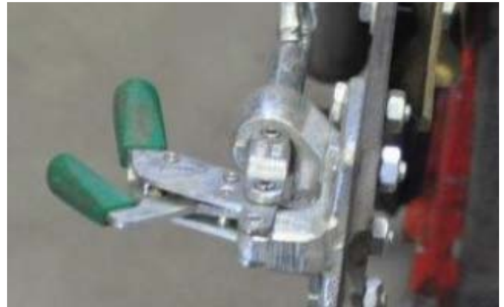
New mechanism to activate mower, replacing toggle switch.
