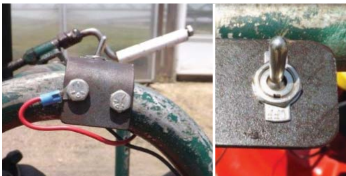
Toggle switch used to activate modified mower.
